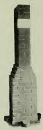
Portland cement mortar and tested when two and a half months old, failed in the smaller portion under 3,540 lbs. per square inch, the stress on the base section being 833 lbs. per square inch. In this case the difference between the upper and lower sections was too great to secure the effect discussed in the preceding paragraph.
