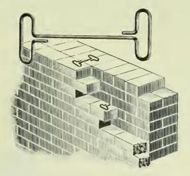
for bonding pressed or enameled brick facings, hollow walls, terracotta blocks, etc., which will, we believe, find favor among architects and builders as being practical and valuable. The claim is made that, being perfectly flat and the formation such, — without spring, — they form a direct lock that bonds perfectly. The accompanying illustrations give a good idea of the exact manner in
