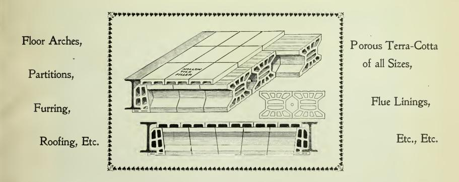
"EXCELSIOR" END CONSTRUCTION FLAT ARCH (Patented).
