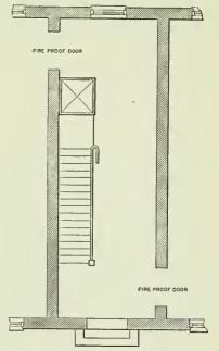
SEPARATING FIRE-STOP HALLWAY, GROUND PLAN.
