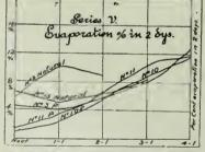
something inherent in the cement itself, which aids it more or less in holding particles of water in suspension. The natural cements show high evaporation neat, so also does the No. 3 Portland, which has a high specific gravity (see general
