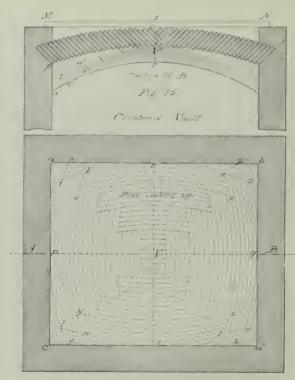
thickness of 0.14 m., and is formed by a single thickness of brick. The backing is of masonry and 0.28 m. thick. The springing line is 3.50 m. above the floor, the wall being 1 m. in thickness, while the thickness of the head walls, which are of adobe, is 0.84 m.
