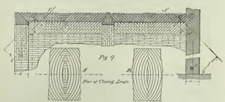
point k to the line of action of T; w' the weight of the head arch, acting through its center of gravity; and z is the width of the head arch.
