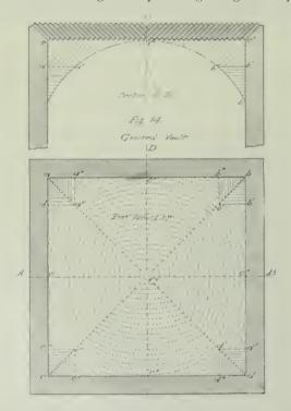
between opposite walls at their middle points and above the apex of the vault, and by two strings p-q and r-s stretched between the vertices of the springing arches a r b-c s d and a p c-b q d. Their points of intersection V, which marks the vertex of the vault, may be made higher or lower by means of the string V'-j attached to the middle of the straight edge M-N, and according to the desired camber.
