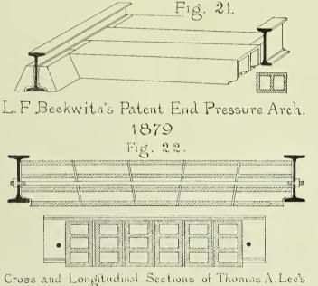
End Pressure Porous Terra-Cotta Arch, Tested at Denver,
