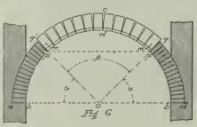
vault, resolved into its two components acting through the center of gravity of the leaf, will produce, first. a thrust parallel to the plane of the leaf and acting against the springing course m-m from
