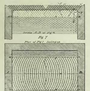
center, or by the method of "vertical leaves." The arch must be strong enough to resist the thrust, and its width is obtained from the equation  $Ts=W_1\frac{z}{2}$  (see Fig. 9), in which T is the thrust of the portion of the vault to the left of the line m" t"; s is the distance of the
