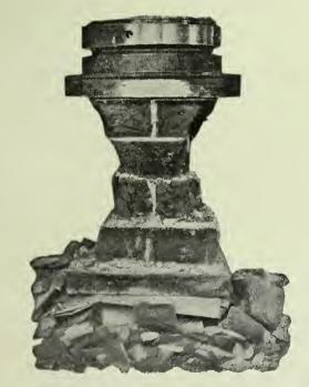
these joints were less than ½ in. thick, the amount of compression in a high brick wall under a load of 80 or 90 lbs. per square inch is seen to be very great, and under a load of 300 to 400 lbs. per square inch, a brick wall 50 ft. high in lime mortar would not only fail, but compress from 2 to 6 ins. in doing so—the compression practically all taking place in the mortar, as in the unyielding Portland cement mortar the compression is seen to be very small.
