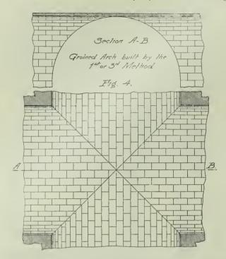
adherence of the mortar and the bricks, which soon form a solid mass and reduce the thrust to a small quantity.
