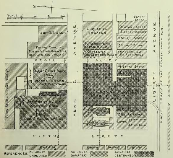
Fig. 1.— Map showing buildings at Pittsburg, Pa., affected by the great fire of May 2 and 3, 1897. The fire started near base of elevator, near center of Jenkins Building, where marked.
