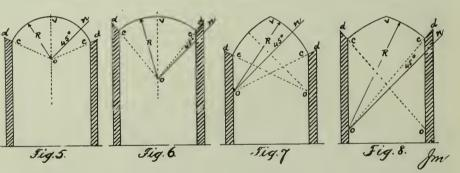
dc inclined planes; o centers of arcs; r radius of arcs; v apex or highest point of intrados; o n the line drawn at an angle of 45 degs, elevation from the center of the arc to intersect the arc or the inner line of supporting pier, as may be.
