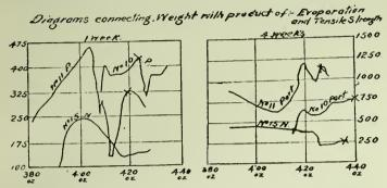
3, except that this product is referred to a uniform section density (i. e.)  $(\sqrt[3]{weight})^2$ ; the diagram is practically the same, showing that the variation in weight of test pieces made practically no difference in the results, i. e., the per cent. of evaporation determines the strength in 1 to 1 mixtures, but is no criterion in neat ones.
