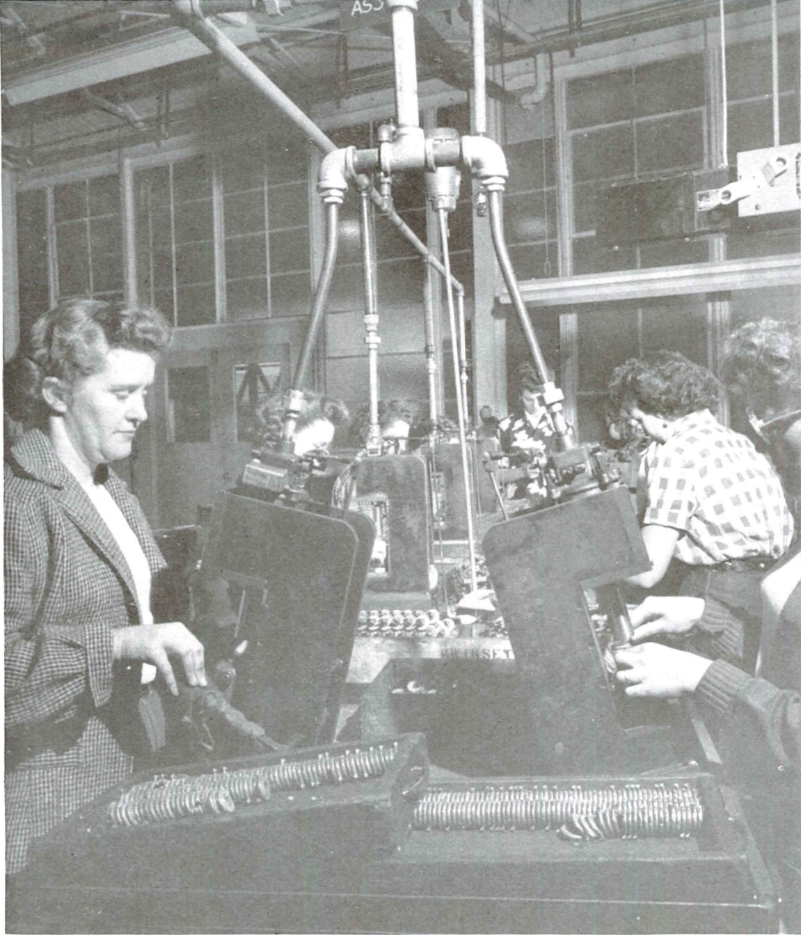
Parts shown at upper left are being assembled here into spindle assemblies.
