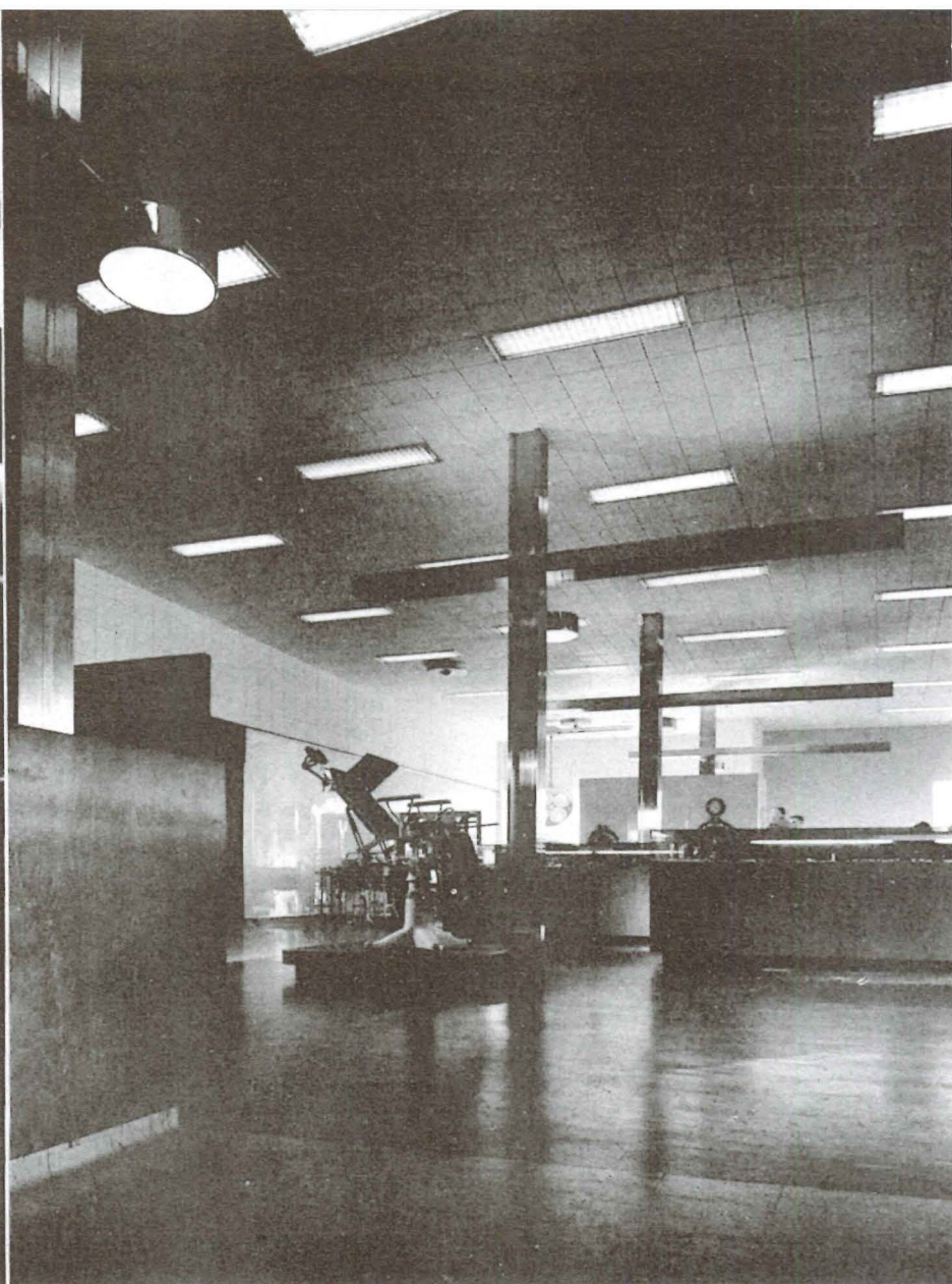
The 10% cantilevering light-troughs and drum fixtures provide indirect and semi indirect light, reflected from the Audioton acoustically absorbent ceiling.
