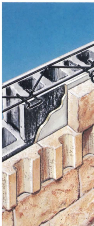
An insulated concrete masonry cavity wall under construction.
