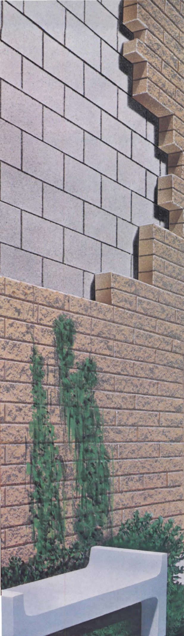
An insulated concrete masonry cavity wall under construction.
