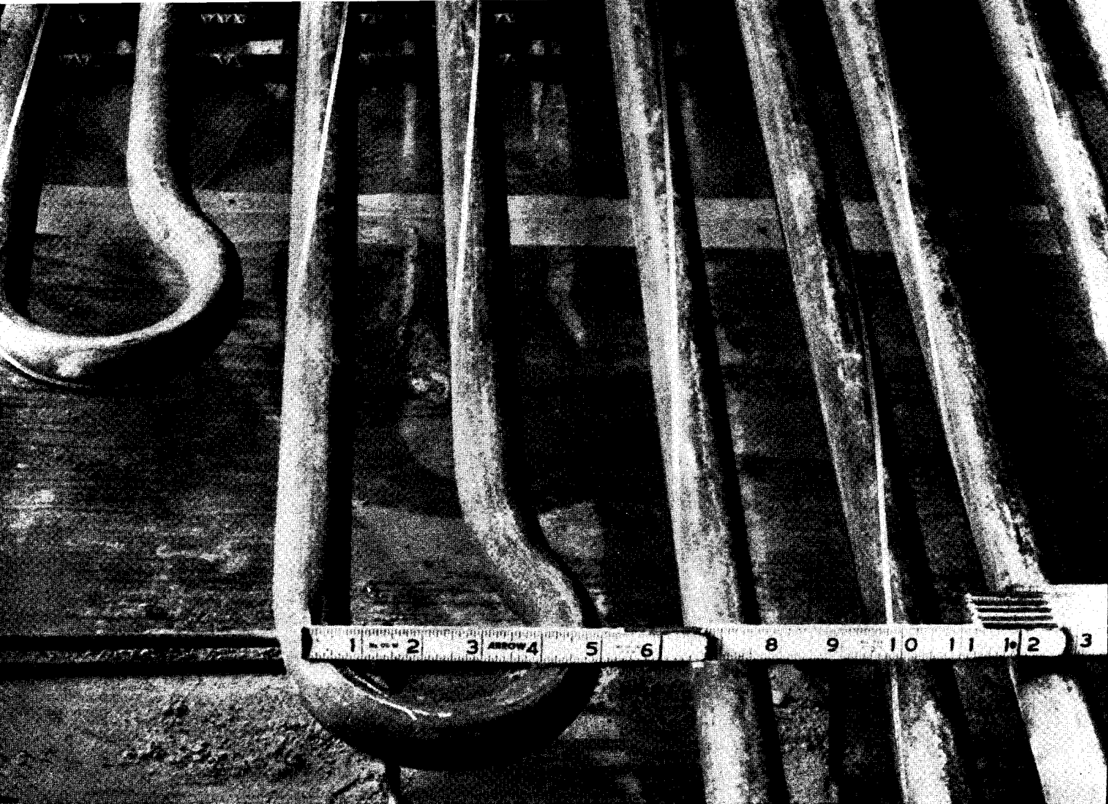
This corrosion resistant 1-inch wrought iron pipe was cold bent to 4½-inch centers.
