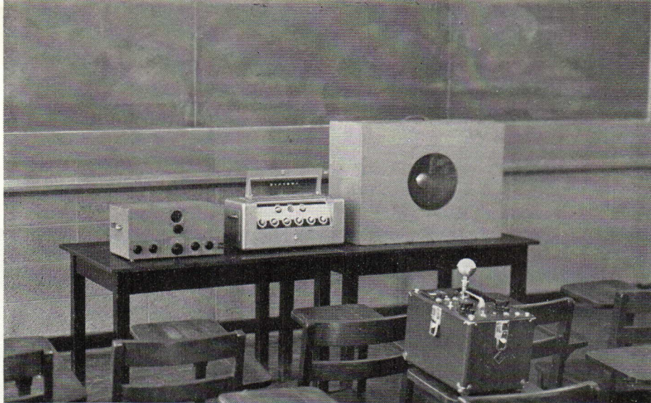
Figure 1: controllable sound source. Equipment shown from left: oscillator (audio frequency), amplifier, and loudspeaker. Sound level meter is located in foreground.
