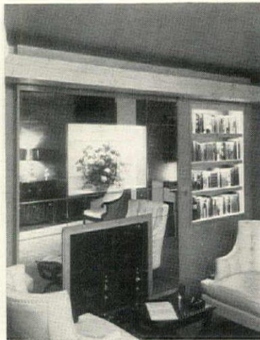
INDIRECT AND DECORATIVE LIGHTING in a living room by Sylvania Electric Products, Inc. Ceiling cove has two continuous rows of 40-watt fluorescent lamps for general light. Shadow box over fireplace uses incandescent bulbs; bookcases are lighted by small fluorescent lamps.
