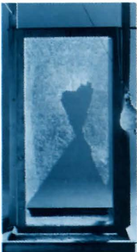
TEMPERED GLASS. This type of glass requires a higher impact energy to break. When it breaks, it shatters completely and the bag passes through it. Only a small number of glass pieces remain in the frame.
