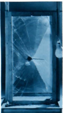
WIRED GLASS. This type of glass breaks similarly to traditional glass with the wire passing through the hole but more pieces of glass stay in place around the point of penetration. Cut wire protrudes.
