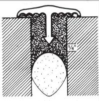
Weathercap's joint protection system is a soft-lead strip embedded in caulk to form a cap or seal for any masonry joint.
