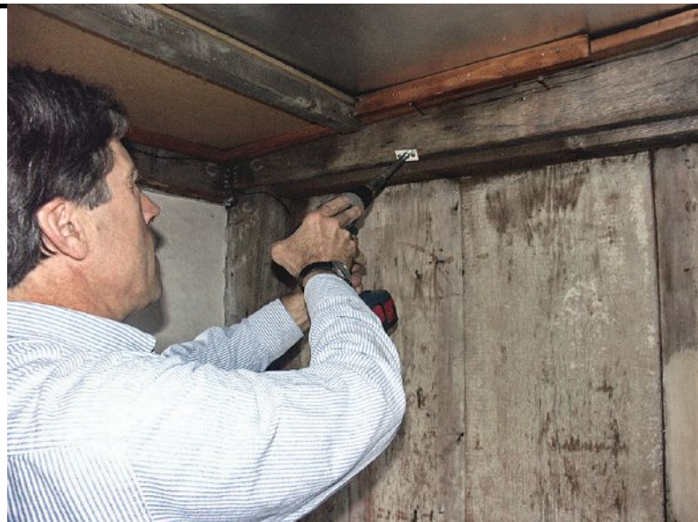
ABOVE: Bill Flynt takes a core sample from an 18th-century chimney girt. Photo: Ed Hood
