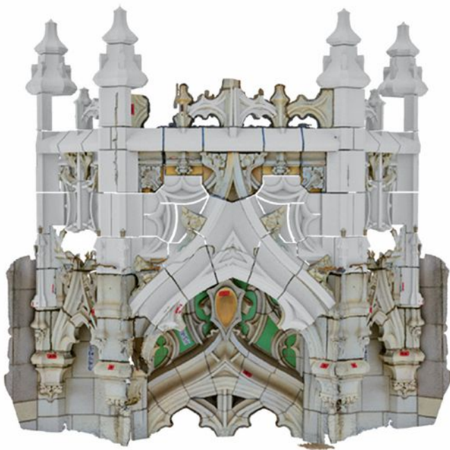
ABOVE: A composite rendering of a section of the Woolworth Building shows replacement terra cotta units created by Boston Valley Terra Cotta draftsmen.
