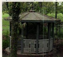
This gazebo features W.F. Norman's Style "A" shingles with its continuous hip finish and a custom-made finial on top.
