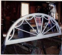
Illingworth Millwork manufactured this attic half-round window sash with spiraled web using single-pane glass and true-divided lites.
