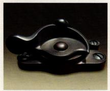
The model LKF18 sash lock from Phelps Company is hot-forged from solid brass and CNC machined; it features a double stainless steel spring mechanism for smooth and positive operation.
