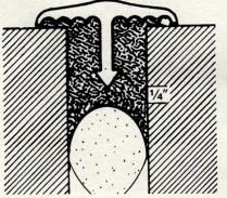
**Weathercap**'s joint protection system is a soft-lead strip embedded in caulk to form a cap or seal for any masonry joint. *Click on* No. 504
