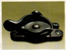
The model #LKF18 sash lock from **Phelps Company** is hot forged from solid brass and hand finished; the internal doublespring mechanism is made of stainless steel. *Key in no. 6001*
