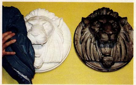
MasterMold, a non-toxic polyurethane paste from Abatron, is used to reproduce molds. Key in no. 1300
