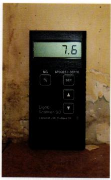
A pinless moisture meter with dual measuring depths of 1/4- and 3/4-in., the Scanner SD from **Lignomat USA** is designed for detecting moisture problems such as dry rot, mold, buckling in wood floors and roofing. *Write in No. 1120*
