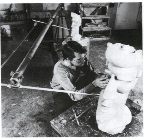
JOHNSON ATELIER is a full-service sculpture studio providing model-making, mold-making, and casting services for architectural elements and sculpture. Shown: Artist using the traditional pantograph method to scale up a model prior to casting.
