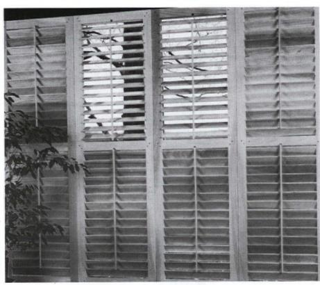
KESTREL MANUFACTURING produced these hardwood, bi-fold movable-louver interior shutters, using blind pocket, mortise-and-tenon construction, with tenons secured in the mortise with through-pegs. Louvers are attached to the louver tilt rod with solid brass threaded eyelets. Write in No. 799
