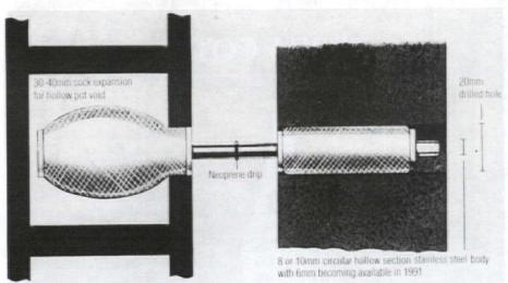
Working entirely from the inside, the sock-and-pin anchoring system from CIN-TEC has been used to re-secure loose terra cotta elements on old buildings.
