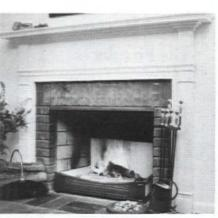
• HearthLight fireplace system supplants log grates; enables wood to burn more efficiently. Decorative cast-iron front panel; back and sides are refractory, and steel pan doubles as a removable ash pan. Company also supplies Ventinox stainless-steel chimney lining system and TherMix insulation, to fill gap between liner and chimney wall. ProTech Systems, 26 Gansevoort St., Dept. TB, Albany, NY 12202 (518) 463-7284. Write in No. 206
