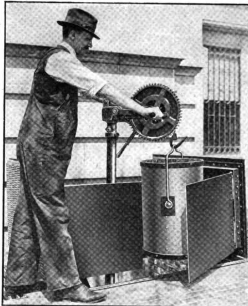
Model A G&G Telescopic Hoist operated by hand power. Operator exerts a pressure of only 12¼ lbs. in raising an average filled can weighing 175 lbs. at a speed of 30 feet a minute.
