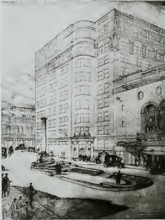
VIEW SHOWING PROPOSED DEVELOPMENT OF THE PLAZA IN THE CENTER OF THE METROPOLITAN TRACT Howells and Stokes, Architects, A. H. Albertson, Associate At the upper end the central feature of the plaza is shown as a shaft of porphyry crowned by an historic Corinthian cap. A quiet fountain is shown at the base and around the outer rim is a small space for gardening. Behind this central feature is a new building, plans for which are being made. This building is to be occupied by one concern. Part of The Arena just completed shows at the left and the Metropolitan Theater is shown at the right.
