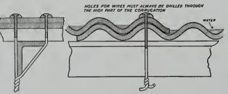
Method of Using Aluminum Wire Fasteners for Attaching Corrugated Ashestos Roofing to Purlins
