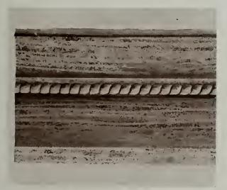
Cast Travertine. Note dark and light veins and granulations.
