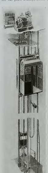
COMPLETE INSTALLATION OF A 1:1 GEARLESS TRACTION ELEVATOR
