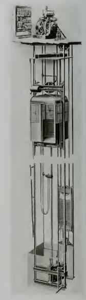
COMPLETE INSTALLATION OF A 2:1 GEARLESS TRACTION ELEVATOR
