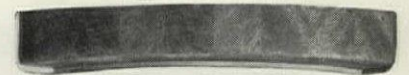
9. Curved plywood angle . . . these photos indicate possibility of standardized series of structural shapes, enormously strong for their weight, nailable, capable of taking a good finish directly on the structural member. . . .
