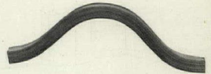
2. The basic material molded when it is created; on edge, this might be a completely self-supporting partition. . . .
