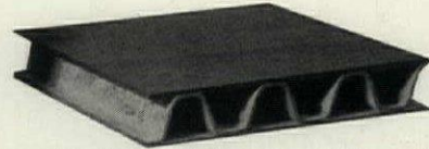
3. Bomber flooring of hollow-cored plywood in three layers, the center one corrugated; approximately an inch thick . . . Implications for building construction?
