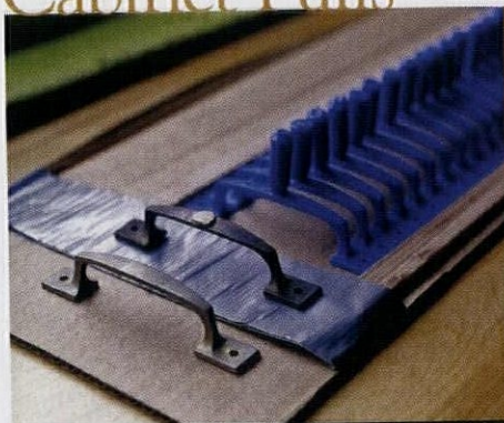
CABINET PULLS were recreated using a lost wax process. Molds (at right) produced rough pulls, which were then polished (at left).
