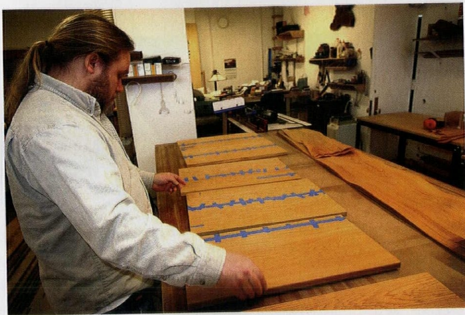
Master carpenter Stafford Norris carefully matches up wood veneer.
