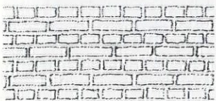
The Dutch cross bond has alternating stretcher and header courses, with every other stretcher course offset.
