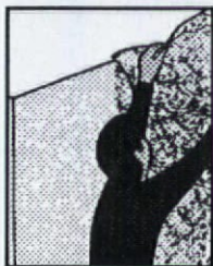
9. Apply mat to 2nd area, overlapping by 1".
