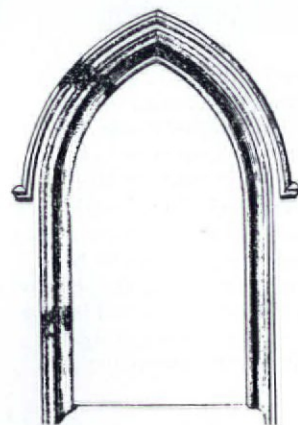
The pointed arch defines Gothic Revival. The lancet arch is narrow, the Tudor arch is wide, and the ogee has two opposing curves on each side. This Tudor arch is from A. W. Pugin's The True Principles of Pointed Architecture . Note the hood mold on top.
