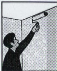
2. Apply saturant to area to be covered.
