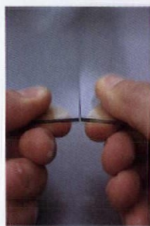
After scoring, bending with two hands snaps the glass.
