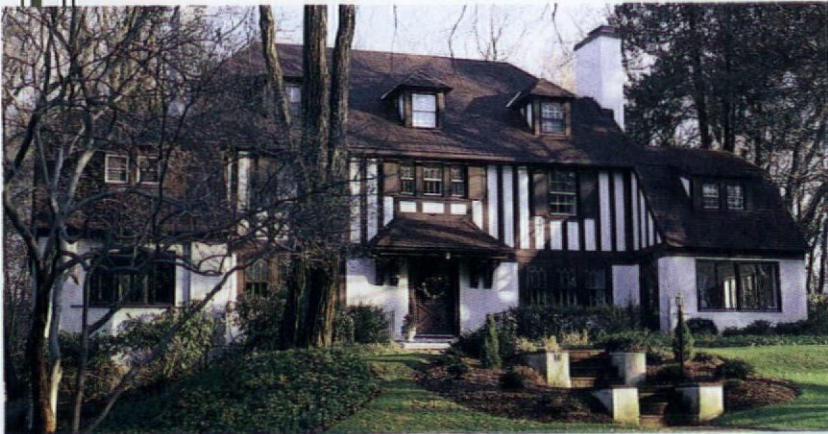
All-vertical half-timbering, here on a home in Summit, N.J., is a common English Revival variant.
