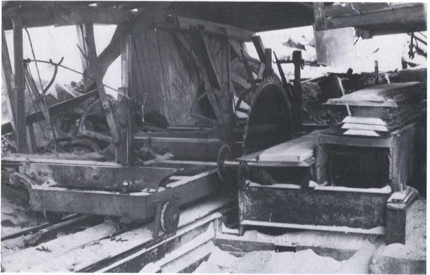
Inside a small, random-length mill. The carriage at left guides the logs through the blade.
