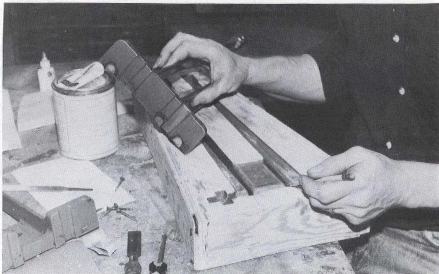
A pattern-maker can re-create a missing piece from a model, or make a unique casting to your specifications.
