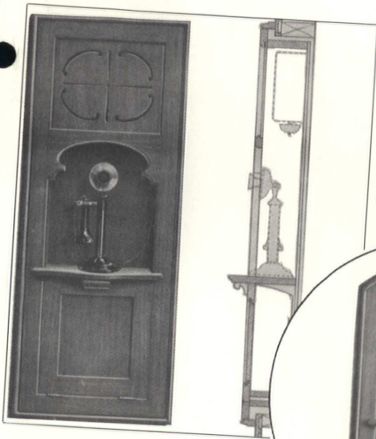
Right: Niches like this one, minus the bell-box panel, were also used to display sculpture or vases. It measures 3 ft. 1 in. high by 1 ft. 5½ in. wide. The wall opening should be 2 ft. 10 in. high and 1 ft. 2 in. wide.
