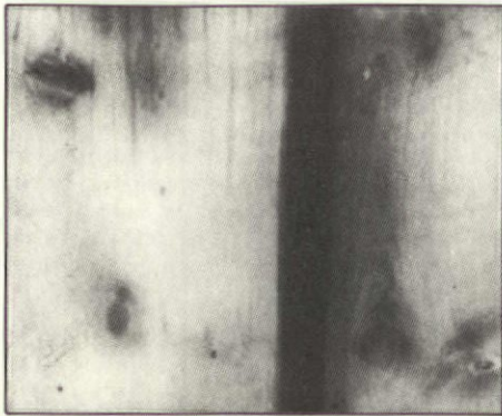
Above: This is the back of a cardboard mount which has been touching a sheet of plywood for years. Materials from the wood migrated to the cardboard, producing this stain pattern.
