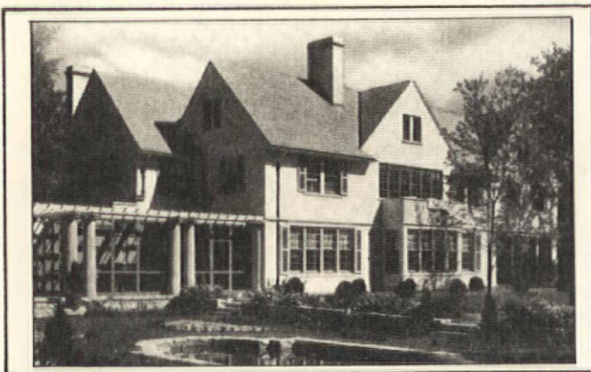
The English Country House Style is a sophisticated and stylized rendition of traditional English vernacular shapes, especially picturesque rooflines pierced by prominent gables. There is usually very little roof overhang. The broad bands of windows in this home recall the fenestration in Tudor houses. The pergola porch to the left is a design idea borrowed from the Craftsman movement.
