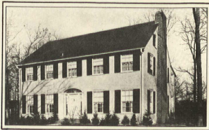
The true Colonial Revival Style was marked by a faithful adherence to the symmetry, proportion and restraint of the 17th century prototypes. This early 20th century house has the symmetry and window placement of a simple early Georgian Colonial house. The doorway, with its fanlight and sidelights, is more characteristic of the later Federal houses.
