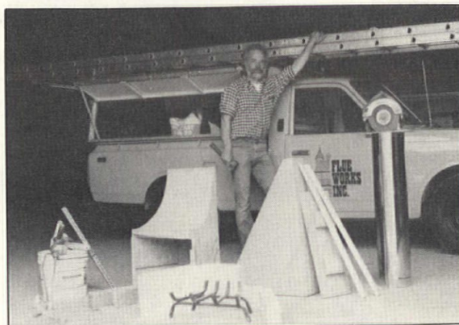
Author Jim Buckley poses with the tools for the job. Left to right: half-inch drill with drywall mixing blade, bucket of refractory mortar, throat form with wooden blocks, firebrick and grate, smoke chamber form with bottom and legs, and 8-in. stainless steel flue pipe with metal-cutting saw.
