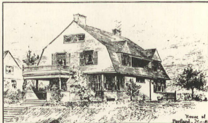
Architect John Calvin Stevens designed this house for himself in 1884. He utilized an all-encompassing gambrel roof to draw in and order the various spaces of the house's main volume.
