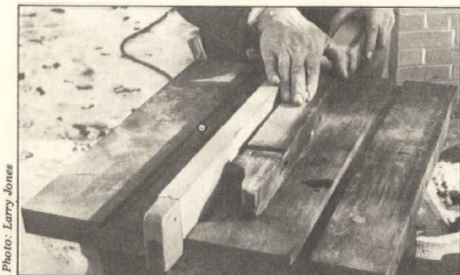
Salt Lake City carpenter Jack Churchill cuts a deeper rabbet into old sash parts. A hermetically-sealed, double-glazed unit will be installed in the reconditioned window sash.
