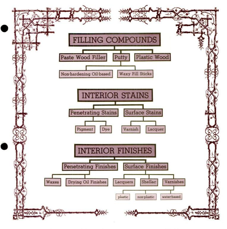
(sometimes alcohol) and an oil-soluble base, both of which are non-grain-raising. Because of their depth of color, dye stains are often used in advance of a pigment stain as a precolor and then treated with the pigment type for colorfastness and durability. In most instances, dye stains are best finished with a varnish system.
