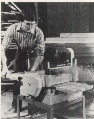
Heavy-duty planer can handle stock up to 13" wide, as thick as 5.9" and as thin as 1/8". Cutter head and feed rolls are raised and lowered with a single handle. Tool is offered with choice of either a 3hp three-phase or 2hp single-phase motor. Rockwell. Circle 405 on reader service card
