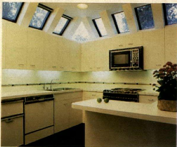
Tilted windows ( above ) provided a solution to a problem: A stable courtyard dating from 1850 provided space to add a kitchen, but Georgetown codes kept Washington, D.C., designer Jeffrey E. Gilbert from putting any windows in walls on the property line. So he glazed inward, giving the room a view of the sky and treetops. Interior design by Thomas Pheasant of Washington.
