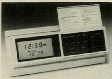
Triple-setback thermostat (above) can be programmed for a week at a time. The "Comfort Zone" unit compatible with standard 24v heat and heating/AC thermostat systems, requires no new wiring when used as a replacement unit. PCI. Circle 246 on reader service card
