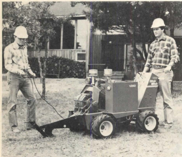
Lawn plow (above) lays cable or plastic pipe with the minimum of dislodgment of soil. The V250 vibratory plow, powered by a 25 hp engine, is capable of installing power, communication, water or natural gas lines, and residential sprinkler systems. Ditch Witch. Circle 407 on reader service card
