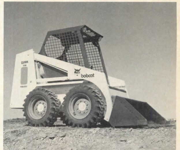
Skid-steer loader (above) has a 1300 lb. capacity. The loader is 75" high and 55" wide for greater maneuverability in confined areas. Unit is available with either a diesel or gasoline engine. All models have a single-speed transmission for smooth handling. Clark. Circle 412 on reader service card
