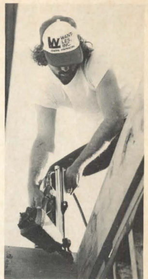
Pneumatic nailer (right) is designed for use in hard-to-reach areas. The heavy-duty CN-325 drives nails measuring from 2" to 3 1/2" long. Duo-Fast. NAHB booth 1961. Circle 408 on reader service card
