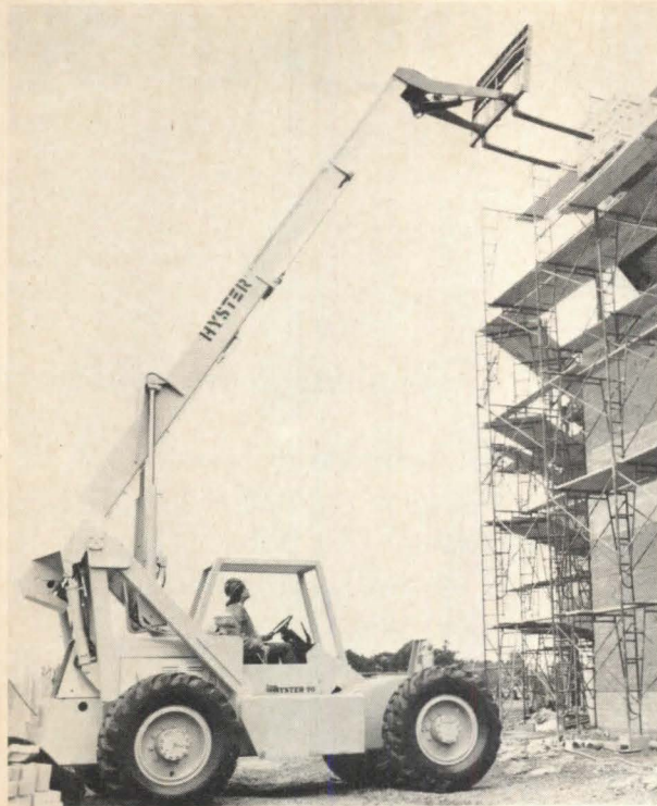
"290A" truck (above) features a telescoping boom and highlift. The boom has a maximum height of 37' and a load capacity ranging from 9,000 lbs. to 2,250 lbs. when fully extended. Hyster. Circle 405 on reader service card
