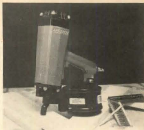
Heavy-duty pneumatic nailer (right) can hold a coil of 300 nails. Tool drives various types of nails up to 2½" in length. An optional attachment allows smooth-shank aluminum nails to penetrate aluminum siding. Tool drives 10 nails/sec. Duo-Fast. Circle 232 on reader service card
