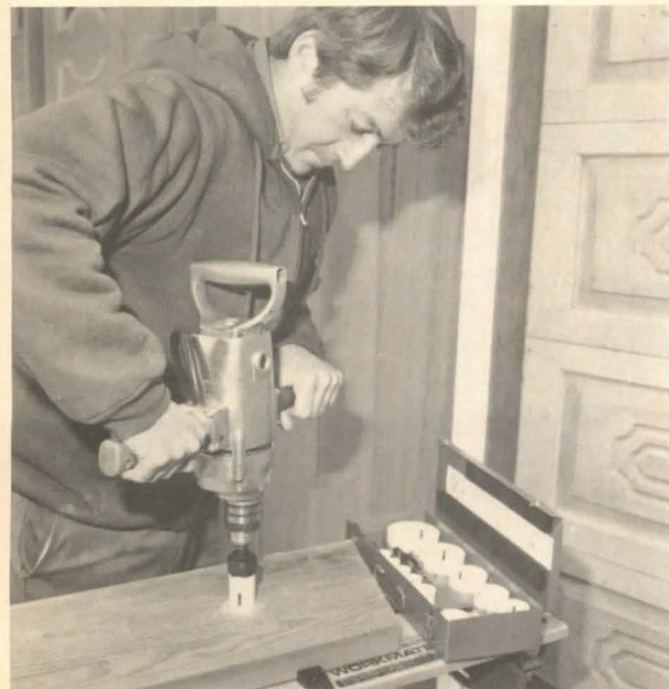
Hole-saw kit (above) includes twelve drill heads, two shafts and three pilot drills. An additional 28 saw sizes are available. American Saw and Mfg. Circle 231 on reader service card
