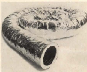
Flexible air duct (above) is composed of an inner air barrier reinforced with a spring steel helix, a layer of 1½"-thick fiber glass insulation and an outer foil jacket. Unit comes in 25' lengths. CertainTeed, Valley Forge, PA. Circle 239 on reader service card
