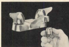
Water-saving outlets, "Econo-Flo" (above) , reduce volume to 1/2 or 3/4 gals. per minute. Units screw into the faucet spout. Outlets are available with male or female threads and in vandal-proof construction. Chicago Faucet, Des Plaines, IL. Circle 248 on reader service card
