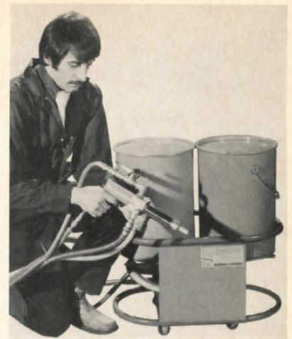
Meter/mix/dispense system (above) can be used to install any two-part fire-resistant silicone foam. The unit holds two 5-gal. drums, positive displacement pumps, two 10-foot-long material feed hoses and a hand-held mix/dispense gun. Sealant Equipment & Engineering, Oak Park, MI. Circle 212 on reader service card
