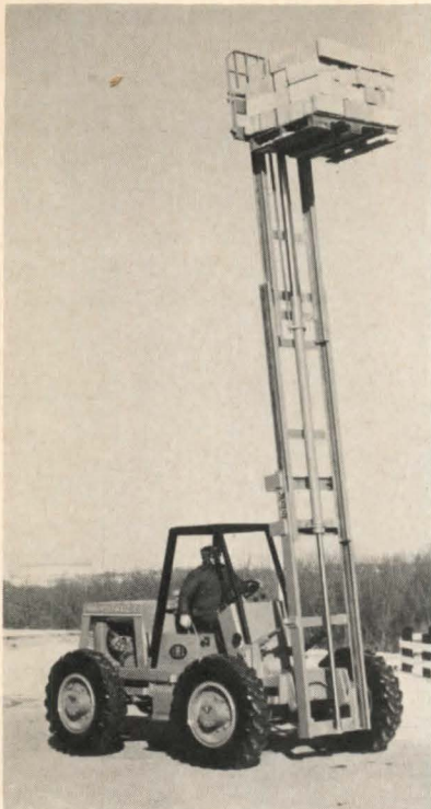
Straight-mast high lift (above) is designed for fast load cycling. Load capacity is 5,000 lbs. at 18 ft. with lift heights to 30 ft. A hydraulic frame tilt for lifting loads vertically on uneven terrain is available. Four-wheel drive and three-speed powershift transmission are standard. Lull, St. Paul, MN. Circle 201 on reader service card
