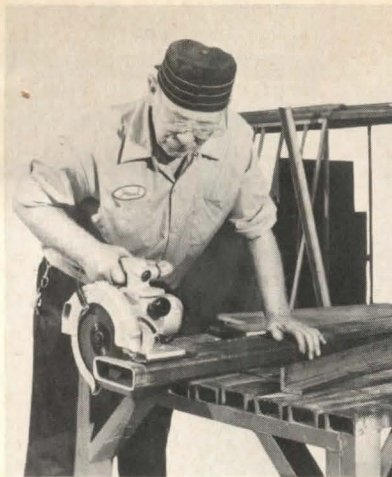
Air-powered circular saw , "Model 74Z-528" (above), is 8¼" wide. The tool cuts through a variety of materials to a depth of 2⅝" and can make angle cuts up to 45° at a depth of 2⅛". A dovetail slide permits the operator to maintain his hand position throughout the cut. Rockwell, Pittsburgh, PA. Circle 211 on reader service card
