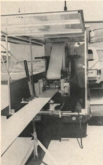
Portable "Siding Factory on Wheels" (above) makes it possible to produce custom-fitted siding on the job site. Steel is run through a portable roll-former, converted to siding panels with a preslotted nailing strip, and cut to a specified length. Seams are thus eliminated. Inland Steel, Chicago. Circle 202 on reader service card
