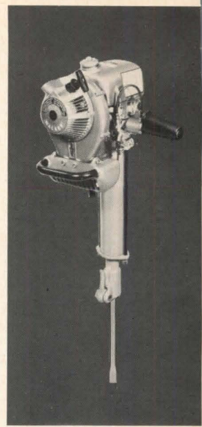
Utility breaker (above) delivers 1300 blows per minute at 35 foot-pounds per blow. Tool is suitable for many heavy-duty applications, including post and sheeting installations. Wacker, Milwaukee, WI. Circle 254 on reader service card
