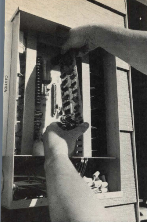
Brains and guts (left) of Energy Programmer are in metal box that's usually mounted outside next to the electric meter.
