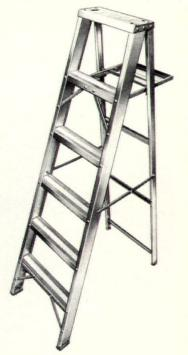
Lightweight Heartsaver® steplad (left) is constructed of heat-trea high-strength aluminum all Steps are 3" wide and serrated non-skid performance. Feet thick nonmarking rubber. Ladde offered in 3' to 8' sizes. White Me
