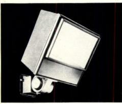
Wall-mounted luminaire (above) permits precise beam-angle control. Cast-aluminum fitting provides field adjustment of 0° to 90°. Housings are constructed in one piece of high-strength, corrosion-resistant cast aluminum. Unit has break-resistant tempered glass lens. McGraw-Edison, Racine, Wis. CIRCLE 240 ON READER SERVICE CARD
