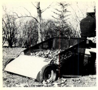
Lawn sweeper with 11-bushel capacity (above) is a two-wheeled pullbehind model. Spot-welded metal sweeper has seven height adjustments including transport position so it can be pulled across gravel. J.I. Case, Racine, Wis. CIRCLE 256 ON READER SERVICE CARD
