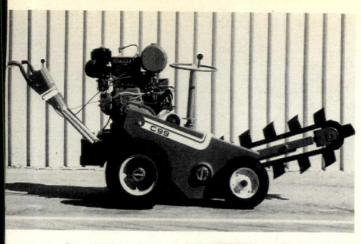
mpact trencher, "C99" (above), dig ditches from 4" to 6" wide 24" deep. Easy-to-maneuver unit tures bolt-on pivot assembly, adtable-height handlebars, wide k cover and heavy-duty bearings. ch Witch, Perry, Okla. CIRCLE ON READER SERVICE CARD
