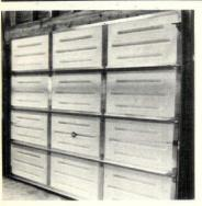
Flush-type garage door, "Therm-O-Air" (above and left), is assembled from extruded aluminum framing and blow-molded polyethylene panels. Double-walled panels with 13/4" captive air space provide thermal and sound insulation, are impact resistant and never need painting. Choice of 3'- or 4'-long panels makes a variety of door sizes possible. General Aluminum, Montgomery, Ill. CIRCLE 237 ON READER SER-VICE CARD
