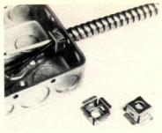
One-piece conduit connector provides for quick, easy attachment of flexible conduits to junction boxes. No tools, set screws or locknuts are required for installation. Heattreated spring steel Tinnerman® connector is vibration absorbing and has a heavy zinc electroplate finish. Eaton, Cleveland, Ohio. CIRCLE 248 ON READER SERVICE CARD
