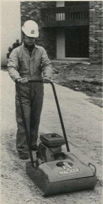
Gasoline-driven vibro plate (above) compacts up to 9000 sq. ft. of granular or mixed materials per hour. "Model VPG 310," powered by a 4.6 hp air-cooled, one-cylinder, four-cycle engine, develops a centrifugal force of 5000 lbs. Low profile, 270-lb. unit travels up to 90 feet per minute. Wacker, Milwaukee, Wis. CIRCLE 264 ON READER SERVICE CARD
