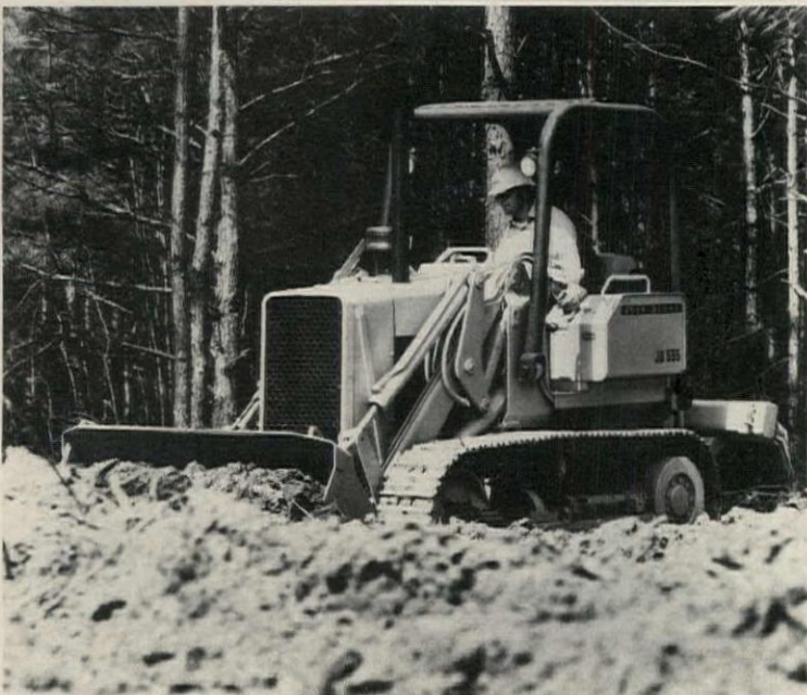
Crawler-loader "JD555" features converter-driven power shift with three forward gears and reverse. Sealed track chains, rollers and idlers, single-level loader control and a 1 1/4-yd. bucket are standard equipment. John Deere, Moline, Ill. CIRCLE 267 ON READER SERVICE CARD
