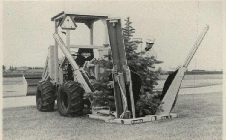
Landscaping/excavating vehicle , "M-437+30," features a four-wheel drive tractor and a tree-moving unit with hydraulically-operated steel spades. Optional attachments include trencher, dozer blade and backhoe/blade. Vermeer, Pella, Iowa. CIRCLE 269 ON READER SERVICE CARD
