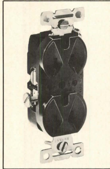
Self-grounding duplex receptacle cuts installation time. The unit is automatically grounded by a copper alloy spring that becomes effective at contact with any grounded metal box. The device, available in 15 or 20 amps, meets NEMA and ANSI configuration standards. Bryant Westinghouse, Bridgeport, Conn. CIRCLE 245 ON READER SERVICE CARD
