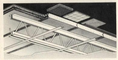
**Floor plank system**, designed for use with steel bar joists, consists of 15"x10' metal-edged gypsum planks. The planks are welded or clipped into position immediately after joists are installed thus eliminating the need for temporary floors. Most flooring materials can be applied directly over sound and fire rated planks. U.S. Gypsum, Chicago. CIRCLE 213 ON READER SERVICE CARD
