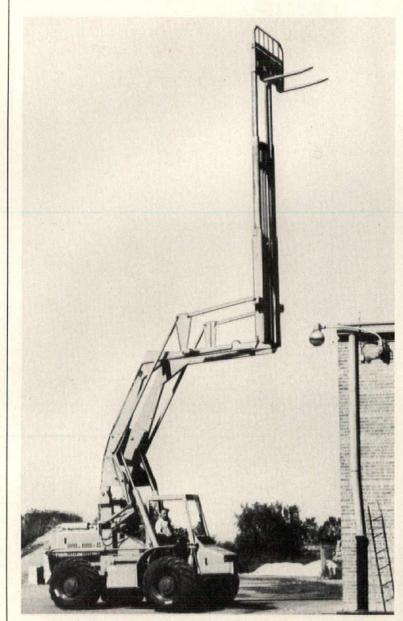
Rough terrain highlift "8000" can elevate a 4,000 lb. load to a height of 42'. The mast has a forward reach of 51" at any height. The heavy duty unit features an oscillation control to assure maximum stability. Teco Crab, Oaklawn, Ill.
