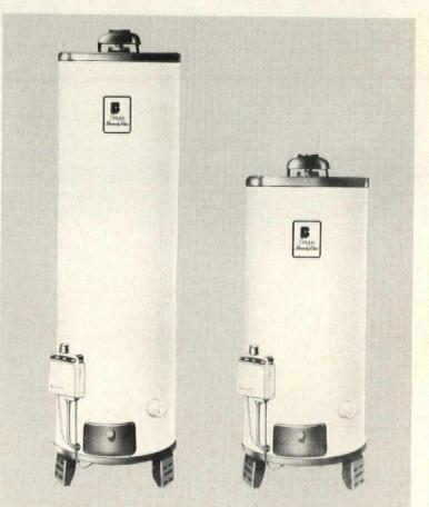
Series of gas water heaters, "BeautyGlas R-GRT-5", offers higher BTU inputs than earlier lines. Offered in regular and shorter "Stubby" size units, the heaters feature glass-lined tanks, safety thermostat controls and gas pressure regulation. Briggs, Tampa, Fla. CIRCLE 234 ON READER SERVICE CARD
