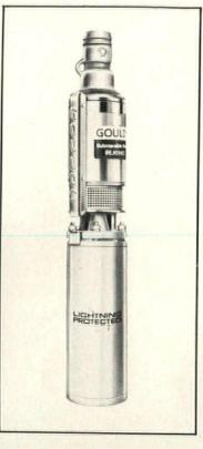
Line of two-wire submersible pumps consists of 31 models suitable for 4" and larger wells. All are powered by Franklin Electric's "Super Stainless" motors with built-in lightning arrestors. Units feature bronze and stainless steel construction, water lubricated bearings and flat bowl design. Goulds, Seneca Falls, N.Y.
