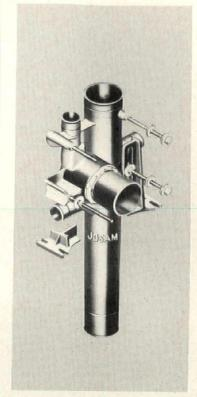
No-hub carrier for use in floor- or wall-mounted water closets eliminates the need for a separate carrier plate. The closet-mounting studs of the "Mod-Stack" are affixed directly into the drainage fitting. Available in 20" and 30" lengths, carriers come with a choice of inlet options. Josam Mfg., Michigan City, Ind.
