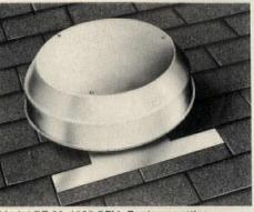
Model RF-68. 1265 CFM. For larger attics. Aluminum housing, self-flashing flange. 7½ changes per hour — 10,000 cubic foot attic.
