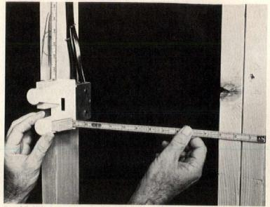
Panel Pal® is designed to measure precise cutouts in paneling and wallboard. Rugged, non-conductive housing unit fits into standard electrical switch or outlet boxes. Then vertical and horizontal tapes are extended and locked into place. Tool is then removed, placed on the face of the panel and used as a template. Toolco, San Angelo, Tex. CIRCLE 248 ON READER SERVICE CARD
