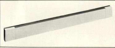
**Draft barrier heater**, designed to provide supplementary heat directly under wide glass expanses, features an architecturally styled ribbon grille top. Heaters with a 188 watt per ln. ft. delivery can offset heat loss from single-pane glass. Berko, Michigan City, Ind. CIRCLE 253 ON READER SERVICE CARD
