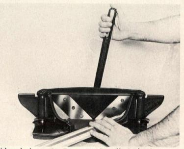
High speed end cutter, "Lion Trimmer", can be used for simple and compound miters, square end planing, bevels, rounds and chamfers. Unit, operating on the sliding knife principle, can be set at any angle between 44° and 91°. It will trim moldings up to 37/8" wide or 5" high leaving a surface that needs no sanding. Pootatuck, Shelton, Conn. CIRCLE 251 ON READER SERVICE CARD
