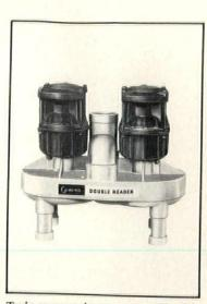
Twin sewage ejector pump, "Double Header", combines two separate pumping units and a common discharge. Utilizing only one pump, the unit has ample capacity for a large house. Should the demand exceed this capacity, or should the unit fail, the second pump starts automatically. Genova, Davison, Mich. CIRCLE 236 ON READER SERVICE CARD
