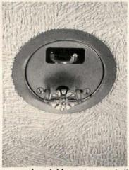
Recessed sprinkler, "Aquamatic," provides fire protection and blends with room decor. Each sprinkler, controlled by heat sensitive bimetallic discs, operates independently. Units will shut themselves off after extinguishing a fire and turn themselves back on if the fire rekindles. Grinnell, Providence, R.I.
