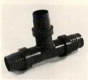
Water line fittings, designed specifically for use with polybutylene flexible tubing, make installation and service of mobile home potablewater lines simple. Solvents, cements and joint-cleaning are unnecessary. Fittings, in coupling or tee configurations, engineered for onsite or factory assembly, use a single-crimp repetitive connection technique. Amp, Valley Forge, Pa. CIRCLE 239 ON READER SERVICE CARD
