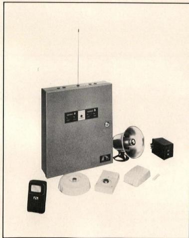
Radio-controlled alarm system is completely wireless. The easy-to-install, "Napcon 3" features window, door and heat sensors and an emergency panic button to signal personal danger. When sensors are tripped, tiny wireless transmitters alert a two-channel alarm system located inside the home. This central unit activates a call for help—a siren and/or a silent telephone dialer. Napco, Farmingdale, N.Y. CIRCLE 207 ON READER SERVICE CARD
