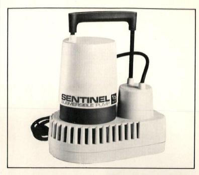
Low-cost, submersible sump pump operates on the vortex principle-a polypropylene impeller spins at 3,100 rpm creating a whirlpool that passes lint and solids without clogging the mechanism. Top-suction pump is actuated by a rising water level. The lightweight unit has a housing of polycarbonate instead of metal. Penberthy, Prophetstown, Ill. CIRCLE 241 ON READER SERVICE CARD
