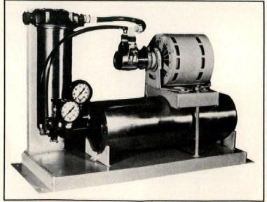
Household-size reverse osmosis water-treatment system reduces dissolved solids by as much as 95% in up to 500 gallons of water per day. The system, which cuts chlorides, sulfates, sodium and calcium, can be adapted to remove iron oxide and hydrogen sulfide as well. It can also be used in conjunction with water softening or chemical pretreatment processes and a water storage tank. Puredesal, Levittown, Pa. CIRCLE 240 ON READER SERVICE CARD
