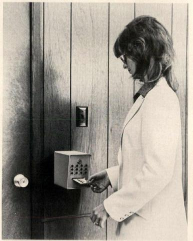
Maximum access control designed for high security areas, Maxcess Controlock, TM incorporates a set of pushbuttons and a card reader that accepts serially encoded magnetic card-keys. Card-key must be used in conjunction with its own personal button code combination. If the wrong code is punched, the alarm circuitry is activated. Lock combinations can be easily changed. Card-key Systems, Chatsworth, Calif. CIRCLE 210 ON READER SERVICE CARD
