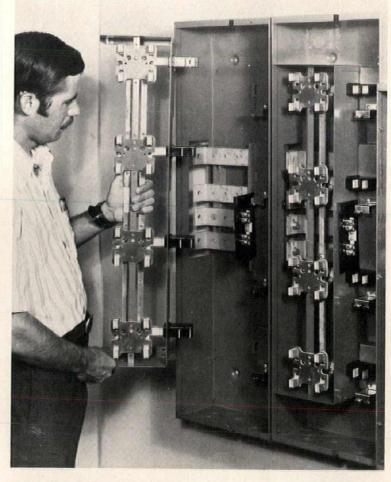
Space-saving stacking meter centers for apartment or light commercial use are easy to install and service. Units can be ordered to accommodate two, four or six 125 amp meters and breakers. Centers feature quick-lift interiors and main breaker mounts conveniently located beside corresponding meter sockets. Bryant, Bridgeport, Conn. CIRCLE 244 ON READER SERVICE CARD
