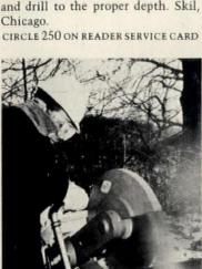
High-speed cut-off saw, "Ripper," can be used on metal, concrete, wood or composition board. The easy-to-maneuver tool features a fast-starting McCulloch gasoline-powered engine. Blade speed is 4,800 rpm. "Engineered Balance" built into the unit provides superior cutting control. Stow Mfg., Binghamton, N.Y. CIRCLE 252 ON READER SERVICE CARD
