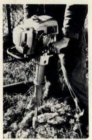
Self-contained utility breaker meets the demands of extended use under punishing operating conditions. The gasoline-driven tool is equipped with a 5 cu. inch, 2.6 hp two-cycle, air-cooled engine. Breaker meets OSHA requirements and features a sound muffler to hold down noise level. Wacker, Milwaukee, Wis.
