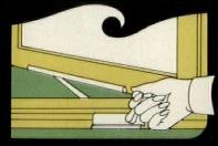
Caradco C-200' Casements swing to a full 90° opening to provide adequate space between the sash and frame to easily clean the outside glass surface from indoors. The neutral tone hardware adds a nice touch of excellence. Crank handle is at a convenient angle for smooth, easy operation.
