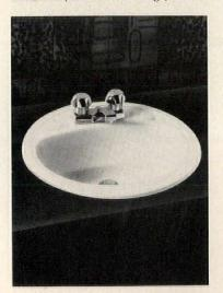
Self-rimming countertop lavatory, "Bayside," is made of acid-resistant enamel-formed steel. The 19"-round unit features a front overflow, two soap depressions and a fitting ledge. It comes in white and six colors. Eljer Plumbingware, Pittsburgh, Pa. CIRCLE 207 ON READER SERVICE CARD
