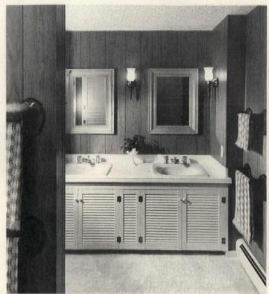
Paneling, with the look of wormy chestnut wood, provides a warm background for a bathroom with an Early American decor. The prefinished, textured hardboard material comes in 16"x8' planks with T&G edges. It installs with wallboard adhesive and simple metal clips. Only damp wiping is required. Marlite, Dover, Ohio. CIRCLE 226 ON READER SERVICE CARD
