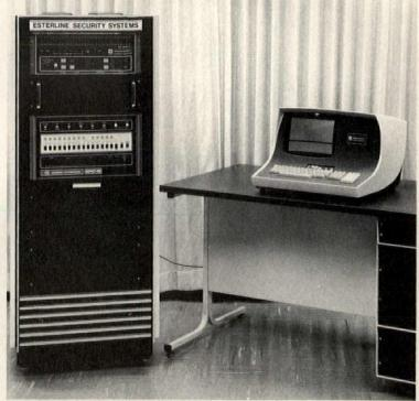
**Security system** provides 24-hour multi-zone monitoring for intrusion, fire, smoke, flooding or other unusual conditions. Utilizing the latest in sensing and data handling equipment, the system scans the sensor network every 3.8 seconds and reports the status of each sensor to a master control panel. Esterline, Costa Mesa, Calif. CIRCLE 217 ON READER SERVICE CARD
