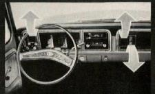
Heater is modern blend-air type; optional "air" is all built in.
