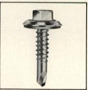
Sealing washer/fastener is for roof or siding applications. Head has a convex underside that produces a ball joint or swivel action on the washer for equal pressure distribution. Metal and neoprene washer resists deterioration. Elco, Rockford, Ill. CIRCLE 211 ON READER SERVICE CARD
